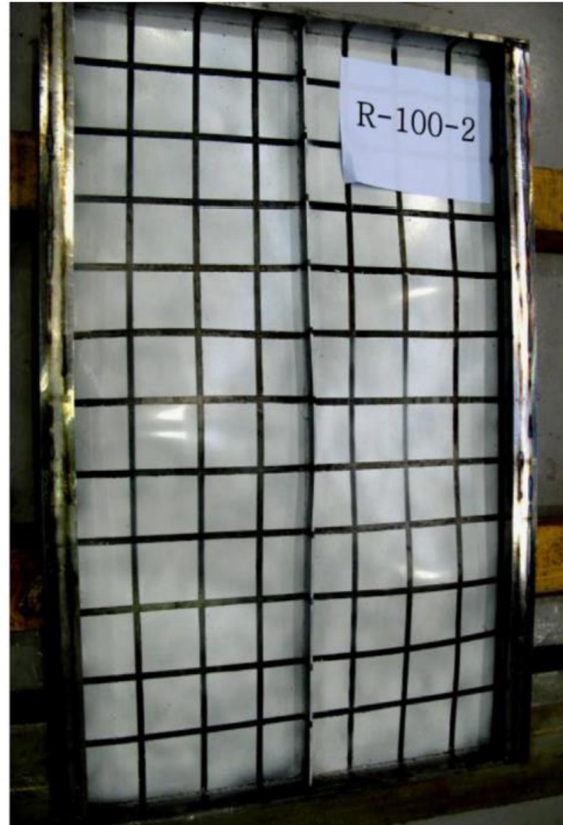
Test setup and deformed shape of the stiffened plate specimen (Kwon, 2014)
